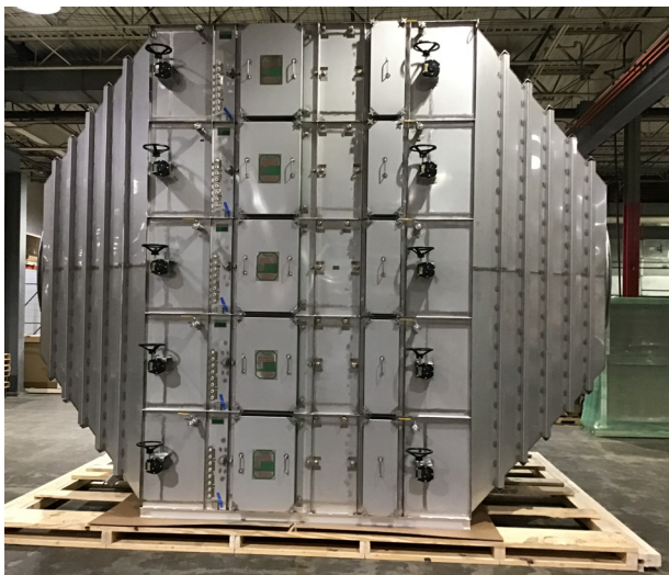
Bag-in/Bag-out containment housing
