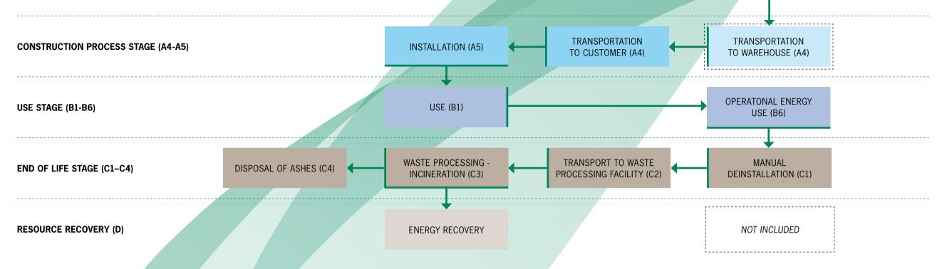
**MODULE A4** covers transportation of the bag filter to the customer. An average transport distance to the customer is assumed to be 350 km and it is representative for year 2021.
